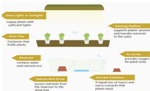
**Figure 1: Hydroponics processes**
