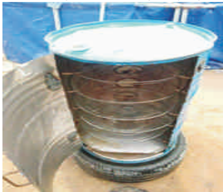
Locally made device from oil drum, processing snails through drying
